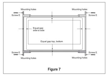
5. Install Air Deflectors top and bottom. Center (left and right) the Air Deflectors above and below the installed BACK FRAME. Secure AIR DEFLECTORS with 4 SCREWS E. See Figure 8. Mark holes and pre-drill the wood cleats with 1/16" drill bit.
